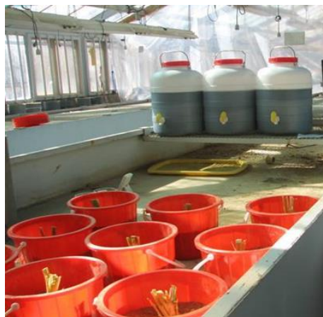
Figure 5. Vetiver watered with landfill leachate with 0%, 20%, 50% and 80% concentrations
